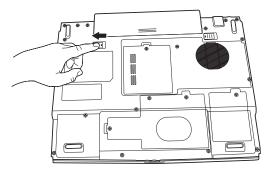
(Sample Illustration) Unlocking the battery release lock
